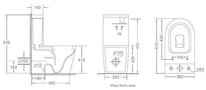
's' trap set out = 100 - 200mm (Finished wall to centre of pipe)
